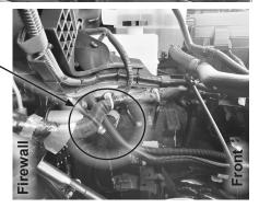
**STEP 2** - Using the image below as reference, release the red locking tab by sliding it to the left. While pressing the tab located on the top right corner of the connector hood, slide the connector hood towards the red tab (to the left) to disconnect it.
